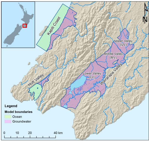
Figure 3: Geographical setting and model domains. Ocean boundaries are simulated with constant heads on the uppermost layer, and groundwater or inactive cells beneath. Outer inactive cells from each model are not shown.
