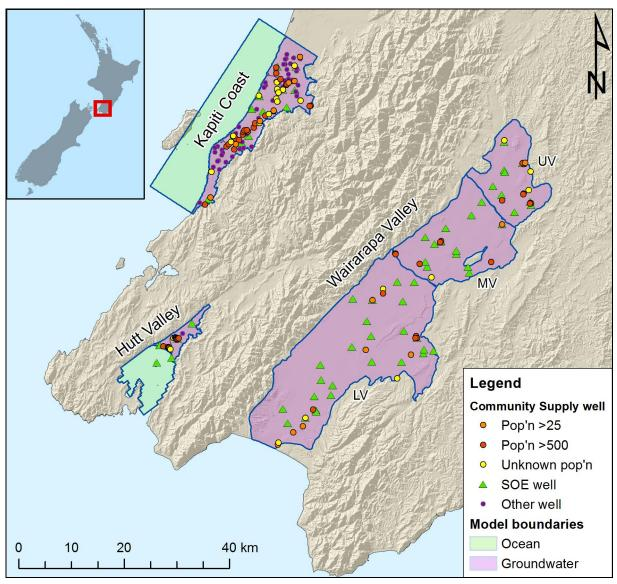
Figure 4: Well locations within the respective model domains: showing community supply wells based on population (pop'n) thresholds, State of the Environment (SOE) wells, and other wells that are not either SOE or community supply wells. Note that some SOE wells are also community supply wells, and have stacked symbols.
