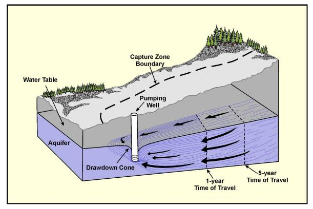
Figure 1: Idealised shape of the capture zone for a well in a homogeneous, unconfined aquifer (modified from Ministry of Environment, British Columbia, 2004).
