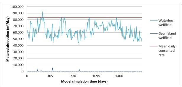
Figure 5: Metered abstraction of the Waterloo and Gear Island wellfield over the simulation period in comparison to the mean daily consented rate over a moving 12-month period (red line). The maximum consented limit (not shown) is 115,000 m<sup>3</sup>/d.
