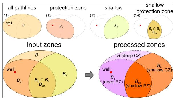
Figure 8: Processing zones from backwards particle tracking results from FEFLOW simulations. Notations used to describe each zone are described in Table 10. In the 'processed zones' subfigure, the four names (in parentheses) and styles are the same as used for maps in the results section.
