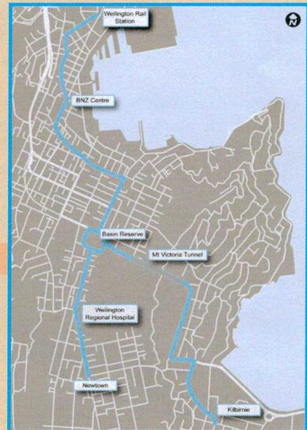
**Light Rail Transit** - Trams running along rail tracks in dedicated lanes with priority signals. Tracks run from the Wellington Railway Station to Courtenay Place. From Courtenay Place to Newtown they run along the median of the road. From the Basin Reserve, trams travel under the proposed Basin Bridge through to Adelaide Road, through a new dedicated Mt Victoria Tunnel and then run alongside State Highway 1 to Kilbirnie.
