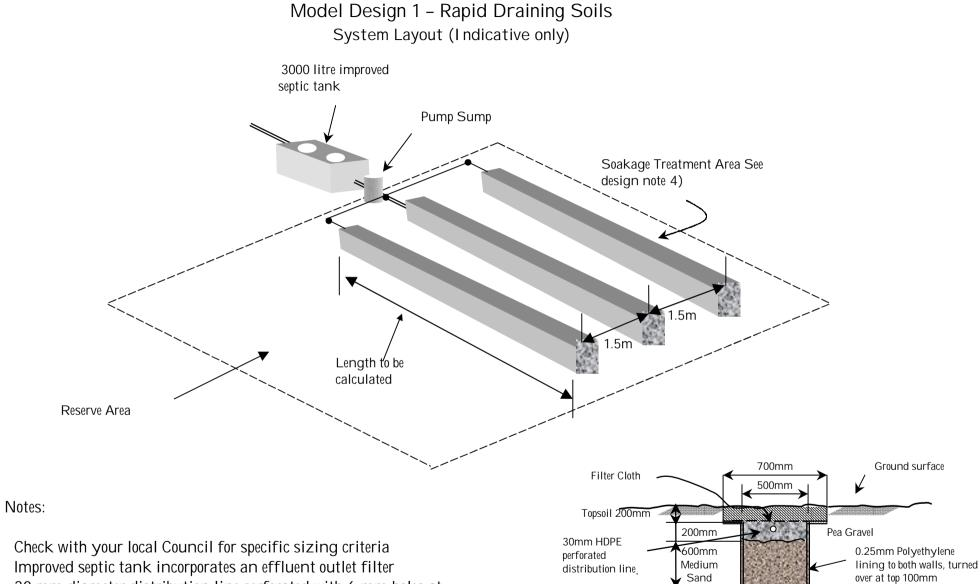
3. 30 mm diameter distribution line perforated with 6 mm holes at 800 mm spacing (design calculations required to confirm)
