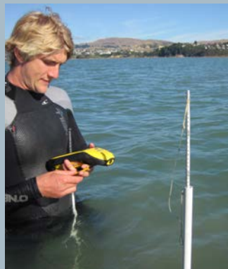
Measuring frame and probe used to measure shallow subtidal plates.
