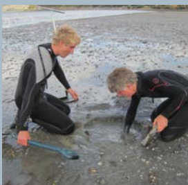
Installing and levelling a sediment plate in Browns Bay, January 2013.
