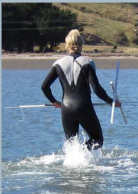
Measuring frame and probe used to measure shallow subtidal plates.
