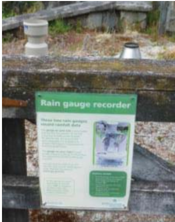
Telemetered rainfall gauge near Morton Dam, Wainuiomata
