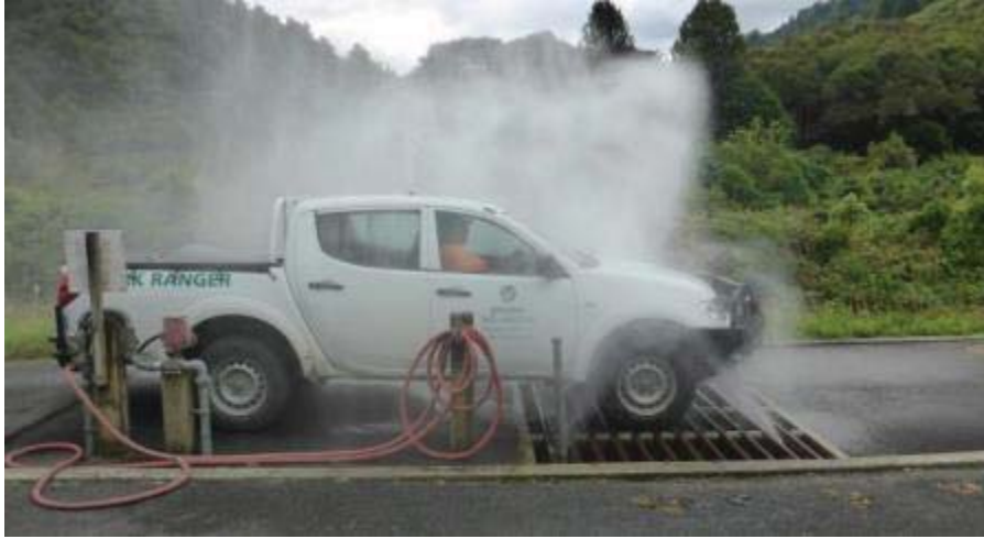
Vehicle wheel wash to remove potential contaminants. All vehicles entering the Wainuiomata /Orongorongo WCA must go through this wash before entering.
