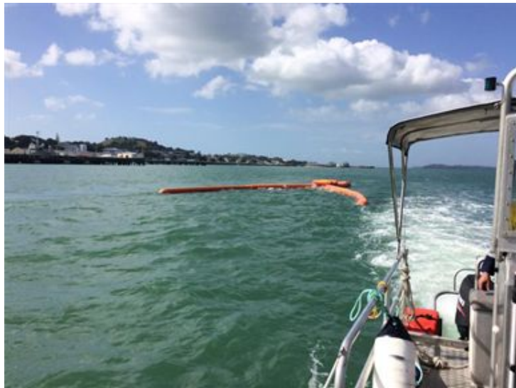
A current buster spill response boom being towed behind a dedicated oil spill response vessel, one of four stationed around the country
