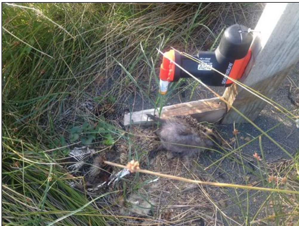
Image 2. Ramp system to allow hedgehog kills to roll away from the trap entrance (Goodnature A24 traps).
