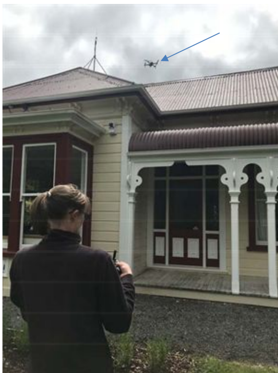
Drone being trialled as a safer alternative for building inspections
