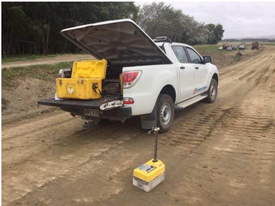
Consultant operating nuclear densitometer for compaction testing on the new stopbank
