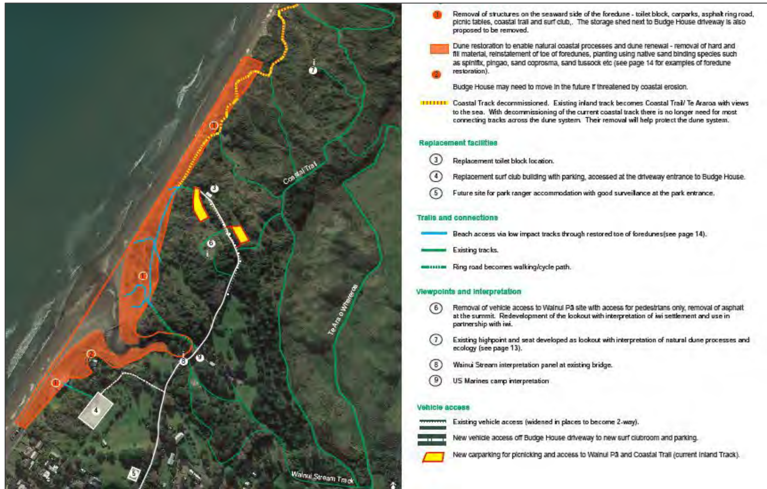
Figure 2: Study area and retreat concept, with area of proposed dune restoration highlighted in orange. (Source – PAOS, 2019).
