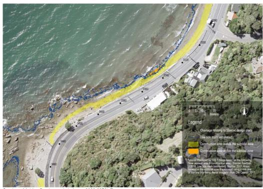
Southern Mahina Bay (around chainage 3330-3370). Treatment type: double curved wall Figure 38 (cont.) Maps showing the five locations where the construction zone may extend into the subtidal zone (orange areas). Low tide level determined by digitisation of aerial imagery by Stantec.
