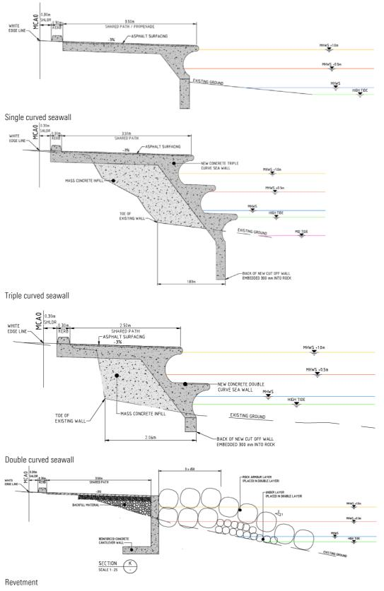
Figure 33 Examples of the designs plans for the proposed wall types for the Eastern Bays Shared Path (Stantec, 2019a) including current and future estimated tide lines for sea level rise of 0.5 and 1m. There will be minor variations on these designs on a site-by-site basis, including the width of the shared path. The tide levels shown are specific to a particular location.
