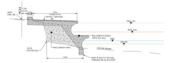
Figure 3-4: Double curved concrete wall
