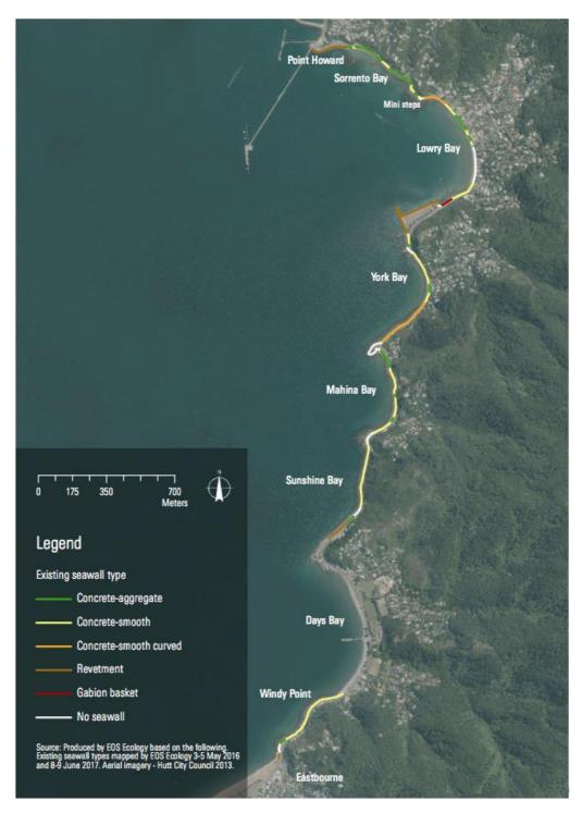
Figure 3<sup>44</sup> Map of the existing seawall types in the Project Area.
