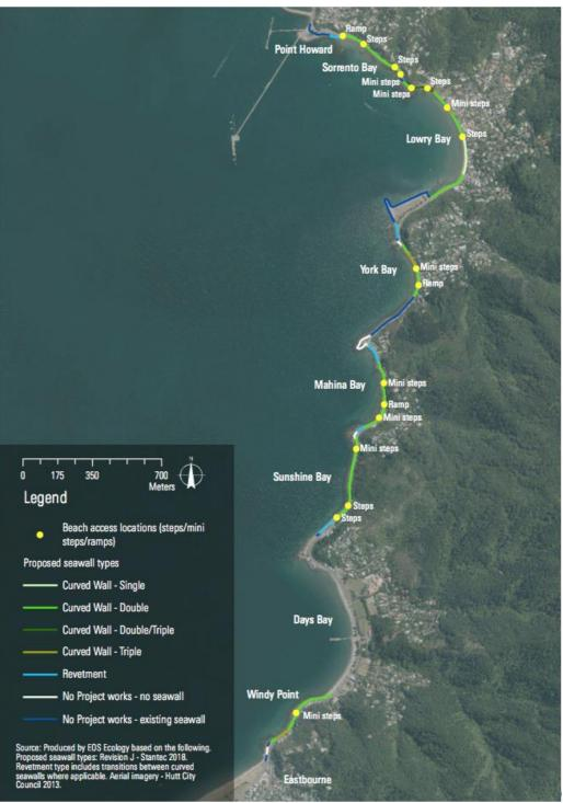
Figure 4<sup>45</sup> Map of the proposed seawall types and access points as outlined in the Revision J Design Plans.
