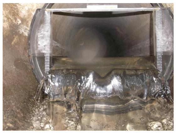
Figure 1 Portable Weir Installed in Featherston Sewer
