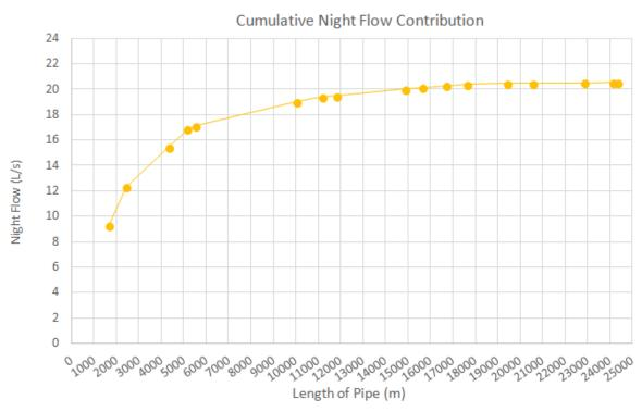
Figure 4 Cumulative Night Flow Contributions (Pipe Length and Flow Rate)
