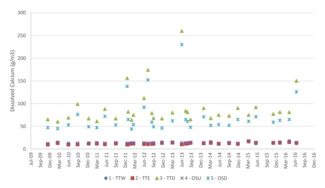
Figure 3-15: Dissolved Calcium for surface water quality monitoring sites.
