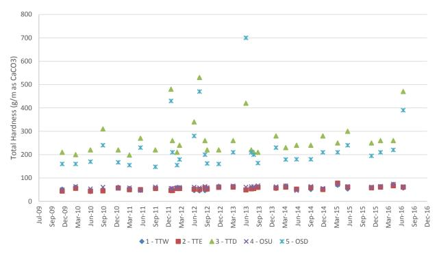
Figure 3-16: Total hardness for surface water quality monitoring sites.
