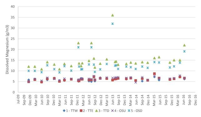
Figure 3-14: Dissolved Magnesium for surface water quality monitoring sites.
