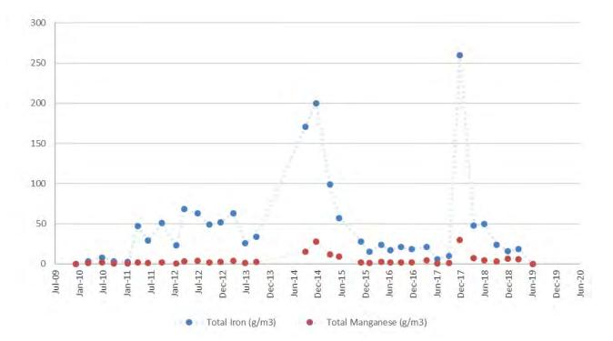
Figure 3-12: Total Iron and Total manganese concentrations in groundwater samples collected downstream of the landfill at site TTG
