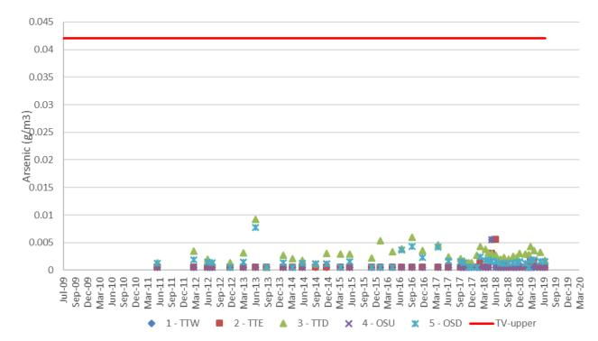
Figure D6: Total arsenic for monthly surface water quality monitoring sites. The red line indicates the ANZECC 90% protection TV as dissolved arsenic V.
