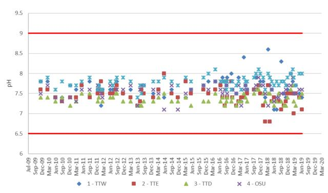
Figure D1: pH for monthly surface water quality monitoring sites. The red lines indicate GWRC recommended guideline levels (Perrie et al, 2012).
