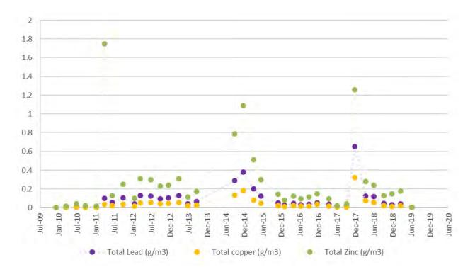
Figure 3-13: Total lead, total copper and total zinc concentrations in groundwater samples collected downstream of the landfill at site TTG
