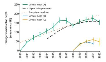
Fig. 2. Change in mean sediment depth over buried plates (±SE) relative to the baseline.
