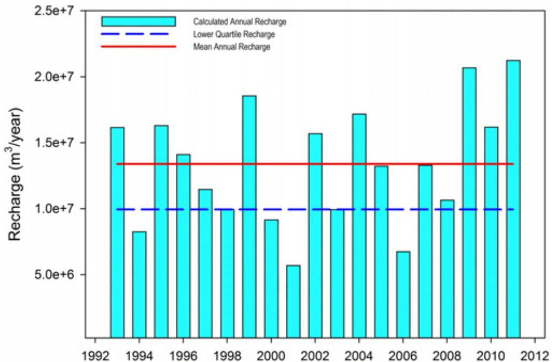
**Figure C2: Modelled annual rainfall recharge (1993-2011) for the Waikanae zone between 1992 and 2012. A mean recharge  $13.4 \times 10^6 \text{ m}^3/\text{year}$  is indicated as is the lower quartile value of  $9.94 \times 10^6 \text{ m}^3/\text{year}$  (dashed line).**
