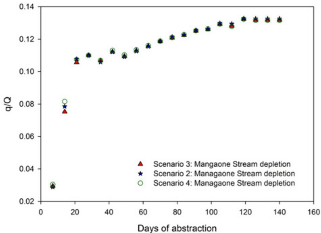
Figure B8: Scenarios 2 to 4 – ratio of surface water depletion (q) to pumping rate (Q) for the Mangaone Stream – abstracting from all the aquifers at 7,500 m³/day (Scenario 2), 15,000 m³/day (Scenario 3) and 20,000 m³/day (Scenario 4)
