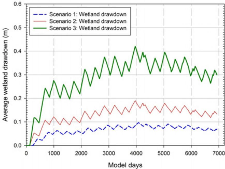
Figure A14: Scenarios 1 to 3 output – wetland drawdowns in the Waitohu zone resulting from pumping an array of synthetic fully screened wells outside Q1 gravels at 3,000m<sup>3</sup>/day (Scenario 1), 6,000m<sup>3</sup>/day (Scenario 2) and 12,000m<sup>3</sup>/day (Scenario 3) for a 19 year model run
