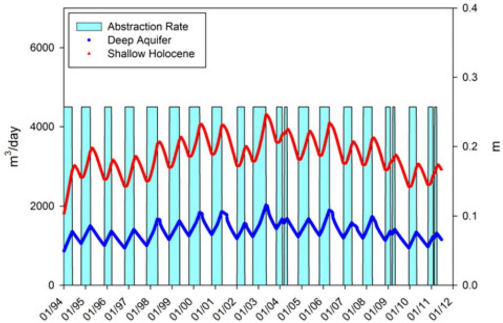
**Figure D11: Simulated drawdown resulting from seasonal abstraction at a rate of 4,500 m<sup>3</sup>/day from the shallow Holocene aquifer and deep aquifer respectively between 1994 and 2012**
