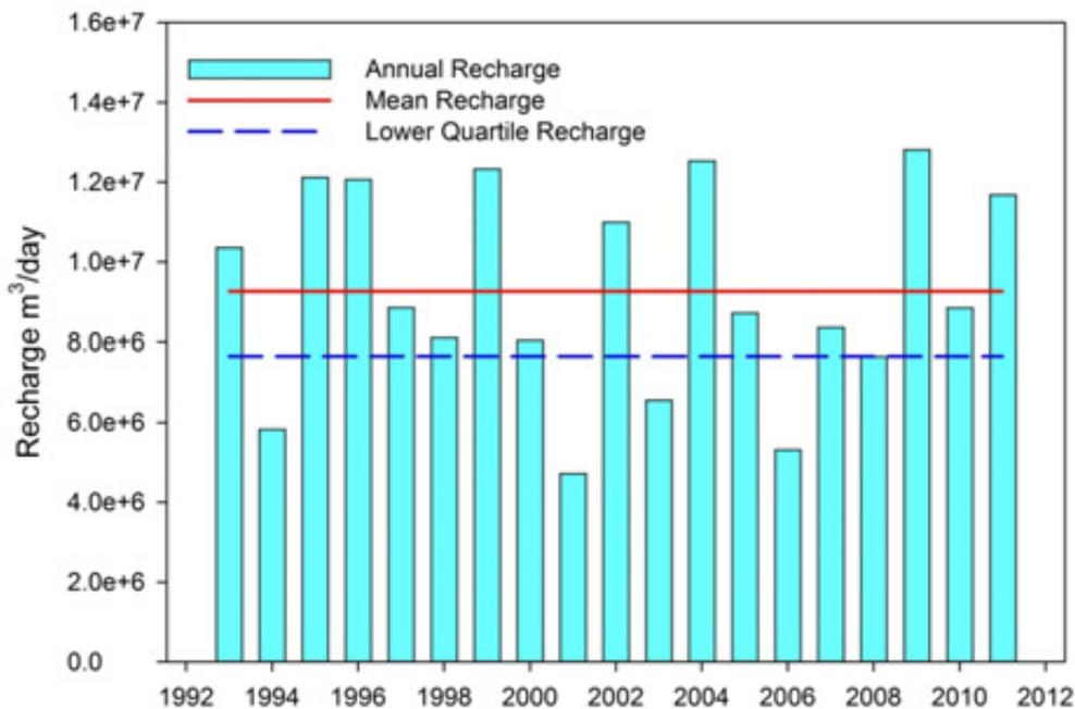
**Figure A2: Modelled annual rainfall recharge (1993-2011) for the Otaki sub-zone between 1992 and 2012. A mean annual recharge of  $9.3 \times 10^6 \text{ m}^3$  is indicated as is the lower quartile value of  $7.7 \times 10^6 \text{ m}^3$  (dashed line).**
