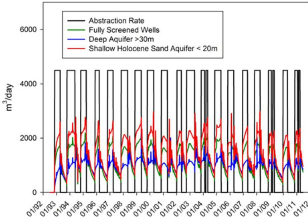
**Figure D8: Comparison of cumulative stream depletion resulting from Scenario 1 (abstraction from the shallow Holocene sands), Scenario 2 (abstraction from fully screened bores) and Scenario 3 (abstraction from deeper bores)**
