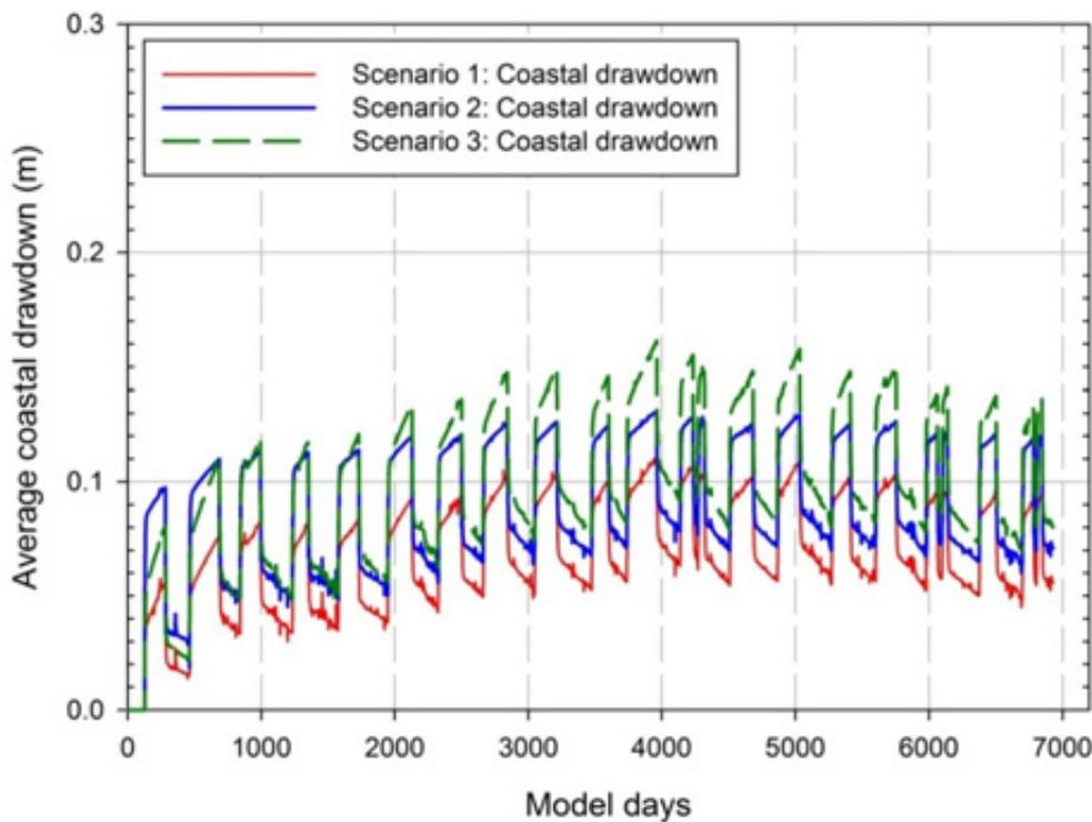
Figure A15: Scenarios 1 to 3 output – coastal aquifer drawdowns in the Waitohu zone resulting from pumping an array of synthetic fully screened wells outside Q1 gravels at 3,000m<sup>3</sup>/day (Scenario 1), 6,000m<sup>3</sup>/day (Scenario 2) and 12,000m<sup>3</sup>/day (Scenario 3) for a 19 year model run
