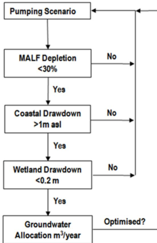
**Figure 4.2: Schematic illustration of the iterative modelling process utilised evaluate pumping scenarios and determine groundwater allocation limits**
