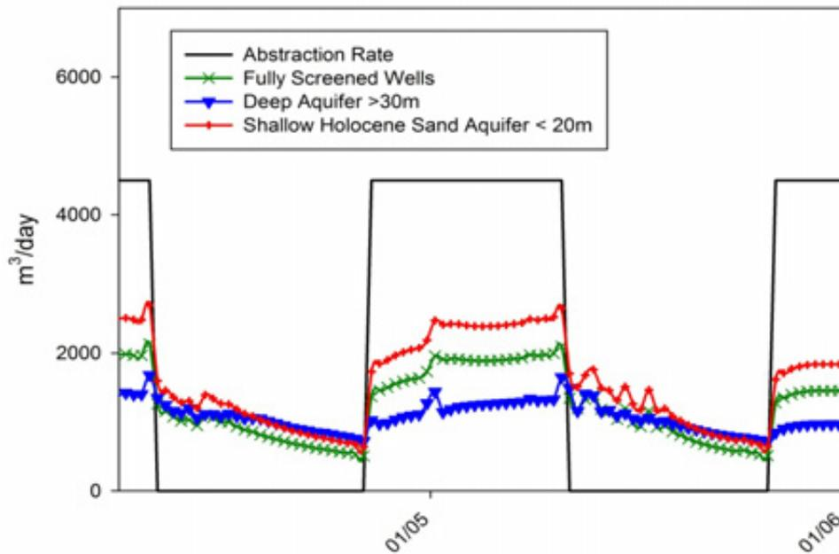
**Figure D9: Comparison of cumulative stream depletion resulting from Scenario 1 (abstraction from the shallow Holocene sands), Scenario 2 (abstraction from fully screened bores) and Scenario 3 (abstraction from deeper bores) over the 2004 to 2006 period**
