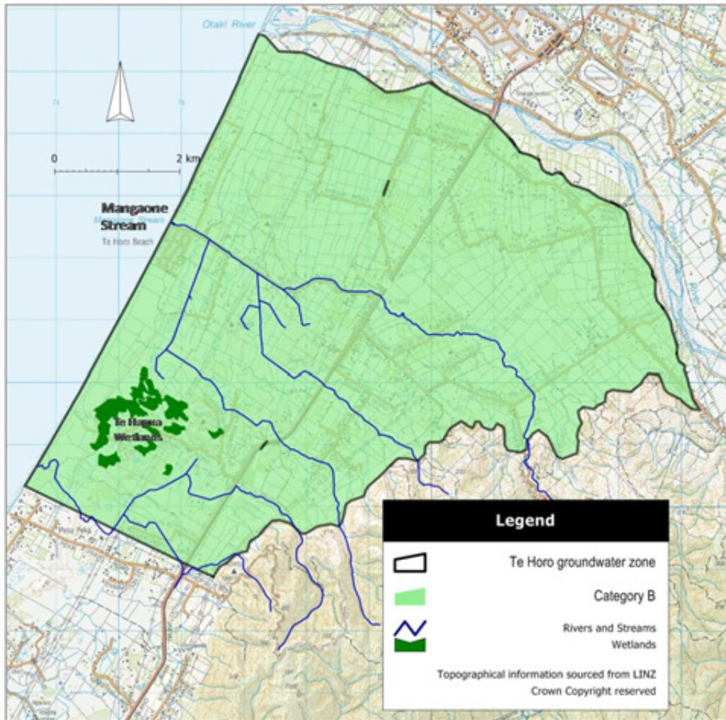
**Figure 4.4: Map of the proposed hydraulic connectivity zonation for the Te Horo groundwater zone showing the location of significant surface water features**
