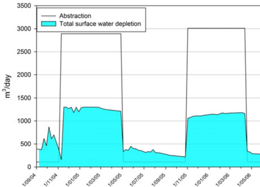
Figure B5: Details of Figure B3 – Simulated historic abstraction and associated surface water depletion in the Te Horo zone between 2004 and 2006. The plot demonstrates the lag between start and termination of seasonal pumping and surface water depletion. Surface water depletion responds almost immediately to pumping. There is a small residual depletion recession throughout the winter which is largely controlled by seasonal rainfall recharge.
