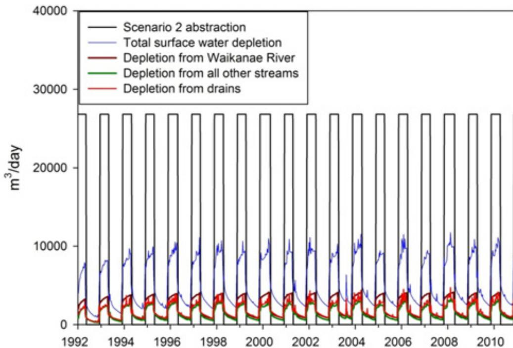
**Figure C10: Scenario 2 output – surface water depletion when pumping from Q6 (layers 6 and 7) only of the of the Waikanae zone. Pumping from current consented bores located in the Q6 (> 60m deep) at an abstraction rate of 26,826 m<sup>3</sup>/d.**
