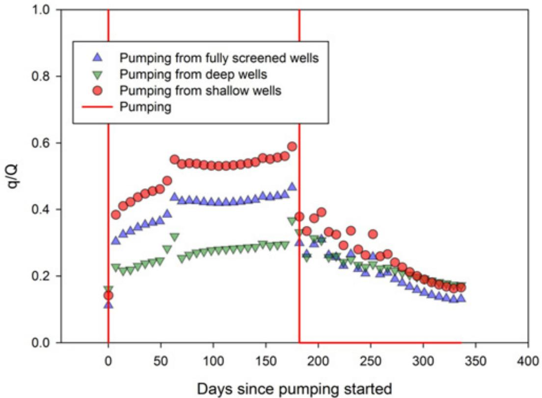
**Figure D10: Simulated surface water depletion after 180 days pumping at 4,500 m<sup>3</sup>/day from the deep aquifer >30m, from shallow Holocene sands <20m and from fully screened wells in the Raumati zone expressed as the ratio of depletion rate (q) and pumping rate (Q)**
